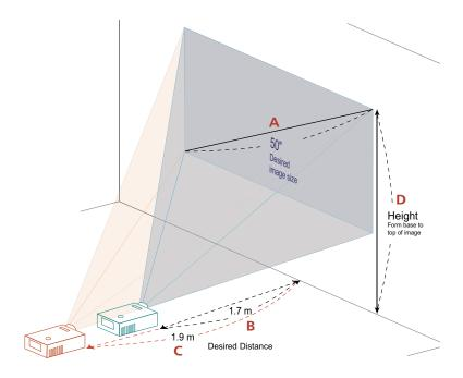
The table below shows how to achieve a desired image size by adjusting either the position or the zoom ring. Example: to obtain an image size of 50" set the projector at a distance 1.7 m and 1.9 m from the screen and adjust the zoom level accordingly.
