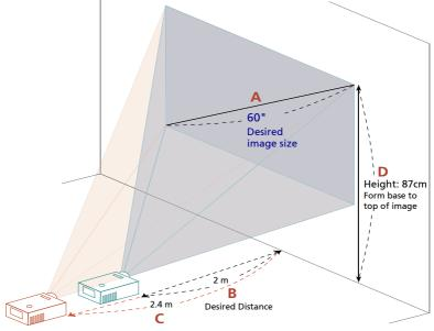
The table below shows how to achieve a desired image size by adjusting either the position or the zoom ring. For example: to obtain an image size of 60" set the projector at a distance 2.0 m and 2.4 m from the screen and adjust the zoom level accordingly.
