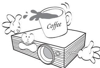
18. Do not place liquids near or on the projector. Liquids spilled into the projector may cause it to fail. If the projector does become wet, disconnect it from the power supply's wall socket and call BenQ to have the projector serviced.
