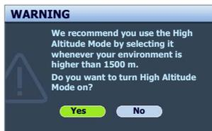
Operation under "**High Altitude Mode**" may cause a higher decibel operating noise level because of increased fan speed necessary to improve overall system cooling and performance.
