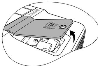
4. Loosen the screw that secures the lamp.
