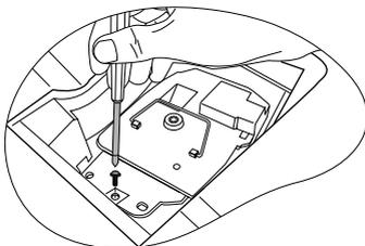
5. Lift the handle so that it stands up. Use the handle to slowly pull the lamp out of the projector.
