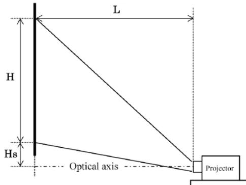
“L” in the diagram (left) represents throw distance. The same image size can be projected with the projector positioned anywhere between the shortest distance L(W) and the longest distance L(T). Here (W) indicates wide, and (T) stands for tele.
