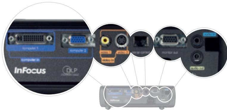
◀ Digital and analog video inputs combine with audio connectivity, RS-232 control and Kensington(R) security.
