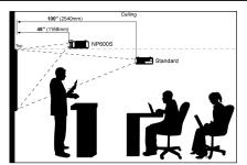
Short throw creates a 77" diagonal image from 3 feet, 10 inches, eliminating shadows on the screen along with projected light in the presenter's eyes created by traditional front projection systems
