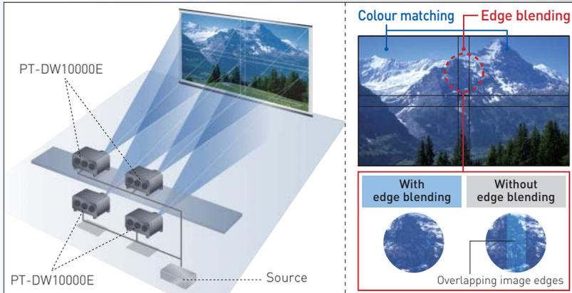
\*When edge blending and colour matching are set, the brightness and colour balance at the boundaries where screens are joined may lack uniformity due to differences in the uniformity of the screen gain directivity, the brightness of each lamp mode, etc.
