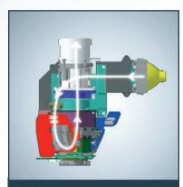
SIM2 ALPHAPATH™ Light Engine: The fundamental feature of SIM2's light engine is its compact structure, which is achieved by overlapping the optical light-path through the engine. This gives it a distinctive ALPHA-shaped appearance.
